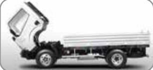
Tilttable Cabin in Any Gear – Ease of Serviceability
